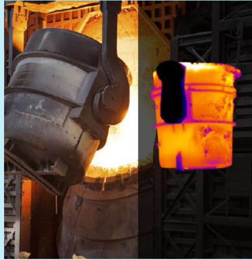
Thermal Monitoring of Refractory Lining
